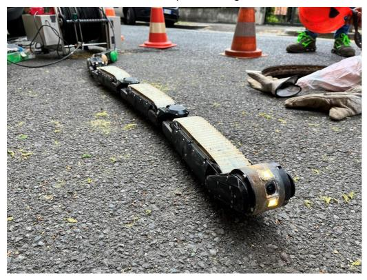
By using Soryu-C, A2A has opened the possibility to efficiently carry out inspection of underground heating infrastructure and also to support the industry decarbonization efforts. Soryu-C, with its flexible design, excels in the inspection of infrastructures that are buried or difficult and dangerous for people to access.
